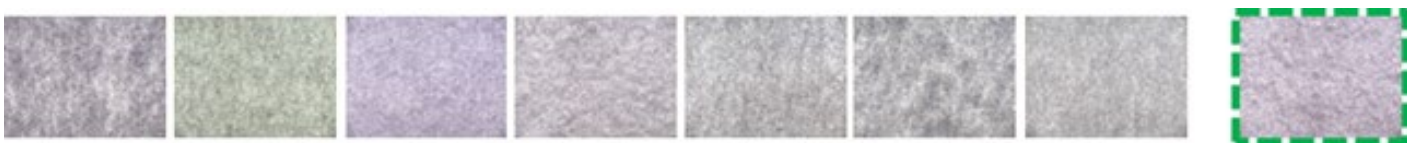
Figure 4. Identification test: Eight types of paper formation images were presented, and the document examiner had to select the image that was most similar to the test specimen (green dotted line).
