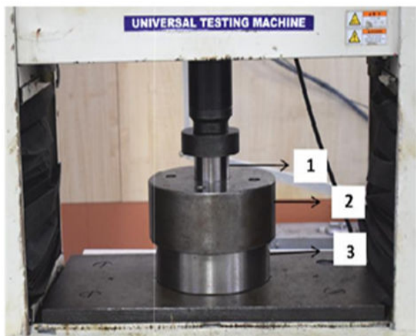
Figure 1. Hole expansion test set up in UTM. Note: 1-Punch, 2-Punch holder, 3-Die holder.
