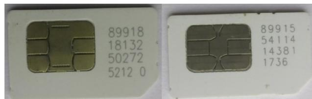
Figure 4: SIM cards showing ICCID.
