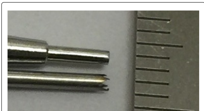
Figure 4: Two different types of surgical punches, one sharp (above) can be used with or without rotation and one serrated (mm scale).
