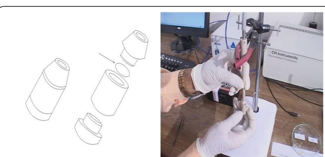
Figure 2: Different parts of fiber optic tip, arrow indicating the position of plastic disc (biocomponent) used for the study, adjustment of disc in the fiber optic tip.
