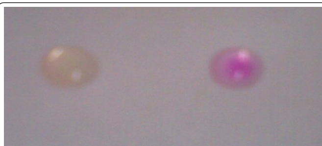
Figure 1: Picture showing the discs (Biocomponent), activity of urease with change in colour i.e. yellowish in absence of urea (left) and dark pink after adding 10 \mu l of 2M urea (right).
