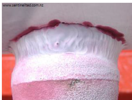
Figure 2: Crack is visible after applying the three sprayers.
