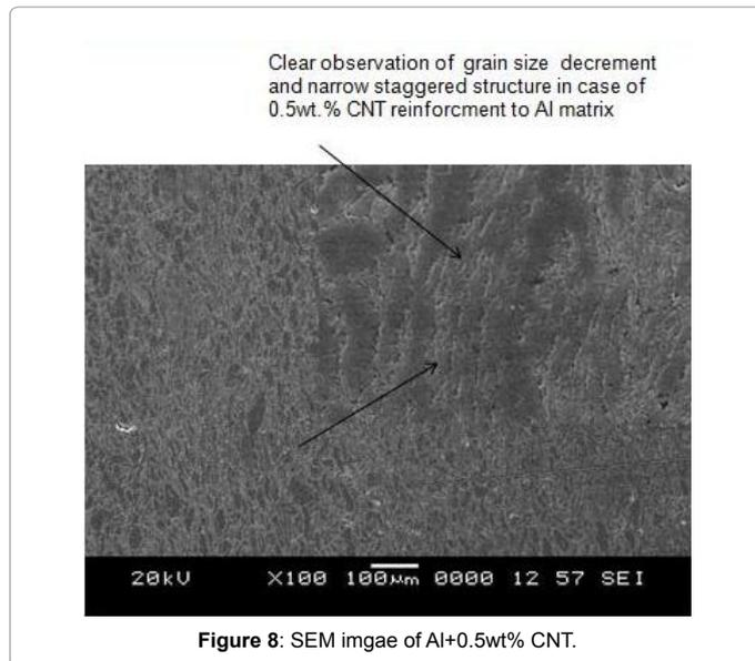
Figure 8: SEM image of Al+0.5wt% CNT.
