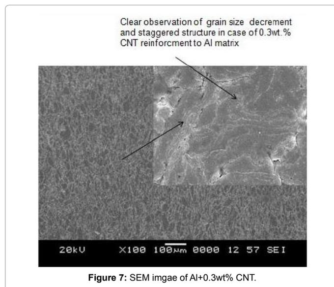
Figure 7: SEM image of Al+0.3wt.% CNT.
