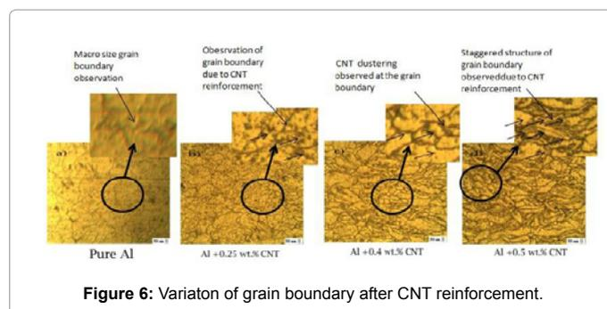
Figure 6: Variation of grain boundary after CNT reinforcement.
