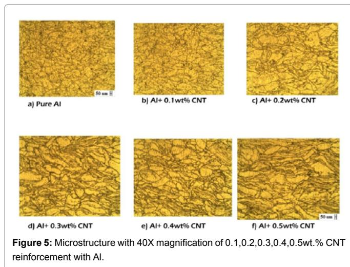
Figure 5: Microstructure with 40X magnification of 0.1,0.2,0.3,0.4,0.5wt.% CNT reinforcement with Al.
