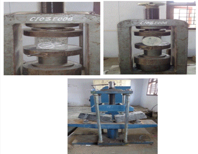
Figure 3: Compressive strength, split tensile strength and flexural strength test of specimen.
