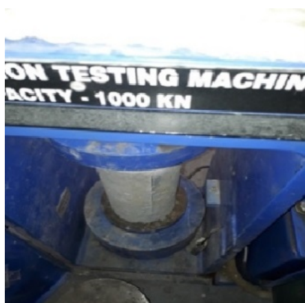
Figure 3: Testing of circular column on CTM.
