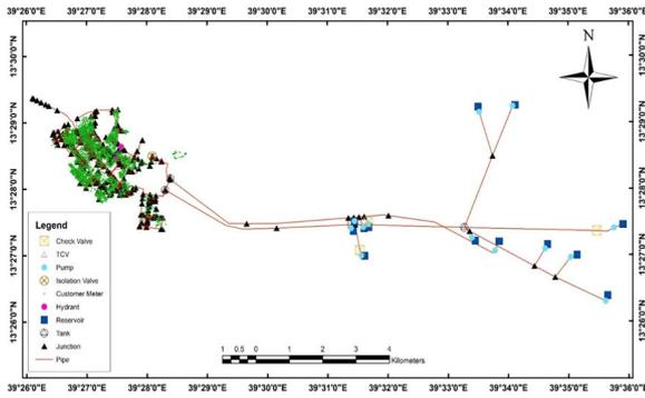
Figure 2. Layout of water distribution network system.
