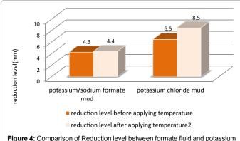
**Figure 4:** Comparison of Reduction level between formate fluid and potassium chloride before and after applying temperature.
