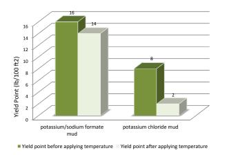
Figure 3: Comparison of Yield point between formate fluid and potassium chloride before and after applying temperature.
