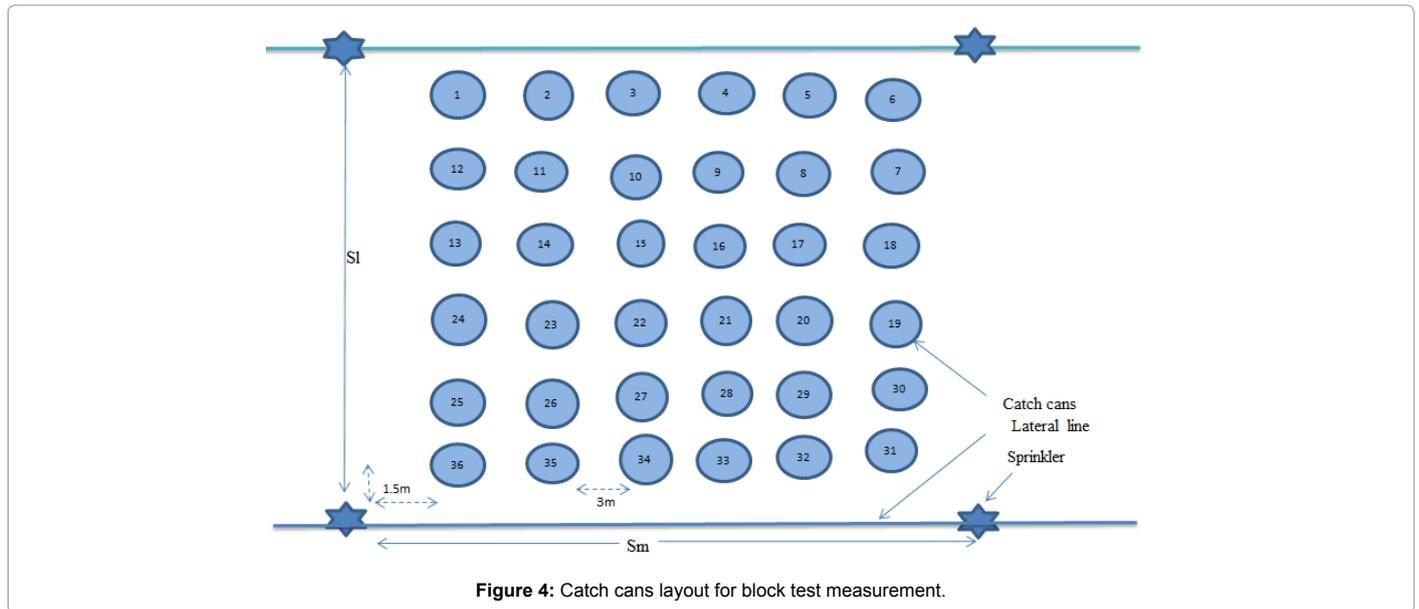
Figure 4: Catch cans layout for block test measurement.
