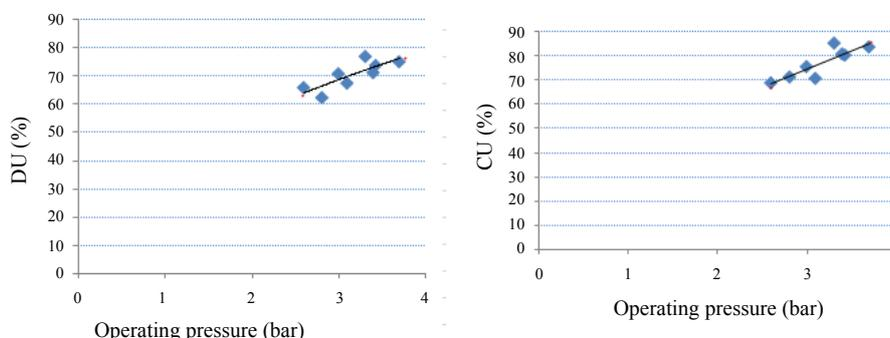
Figure 6: Variation of  $DU$  and  $CU_c$  value with sprinkler operating pressure.
