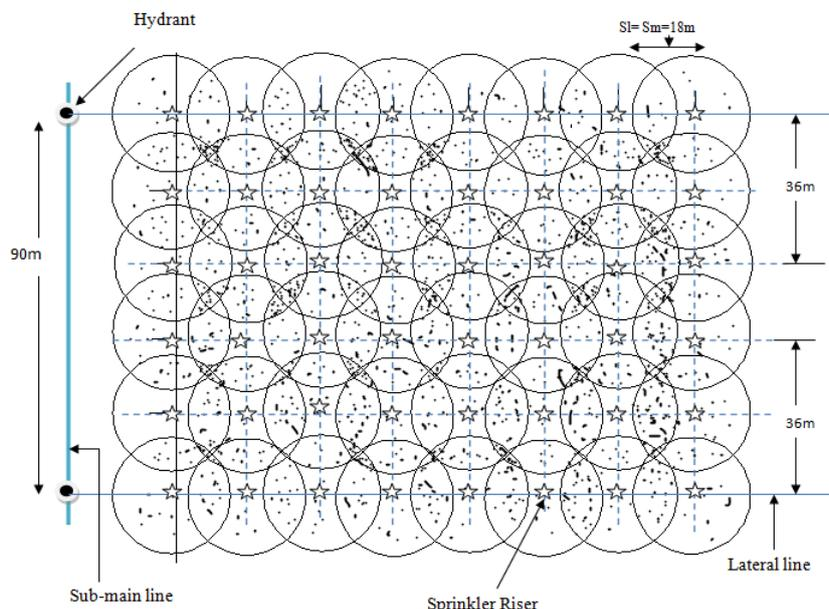
Figure 2: Layout of operating sprinkler irrigation system at Finchaa Sugar Estate.
