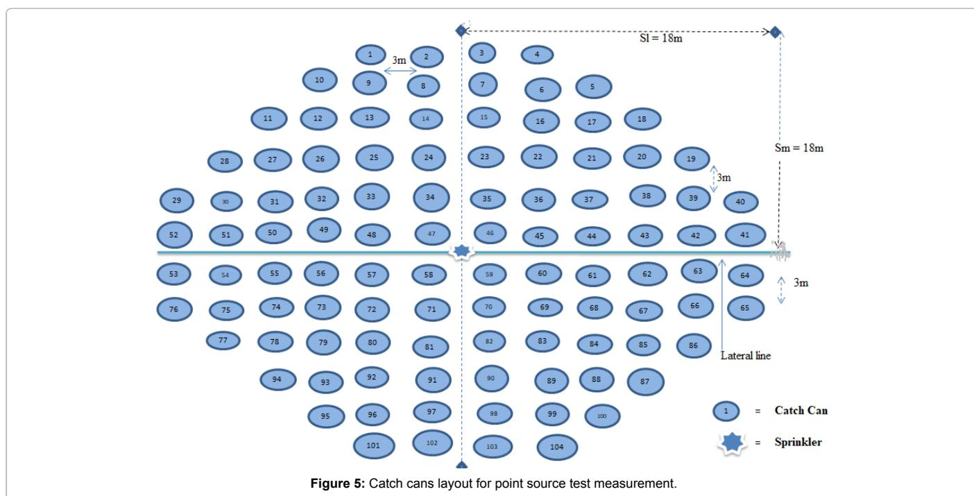
Figure 5: Catch cans layout for point source test measurement.
