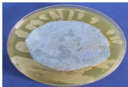
**Figure 1:** Microorganism *S. aureus* Incubated plates for interruption of growth, showing the clear zone around specimens denoting an effective antimicrobial properties according to AATCC 147 – 2011
