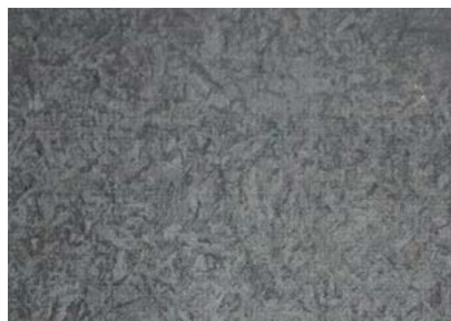
Figure 5b: EN 18 Oil quenched.
