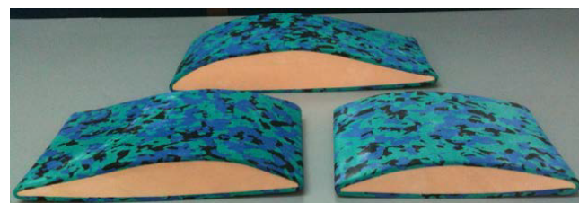
Figure 8: Half- Bolsters used to provide lateral bending moment.
