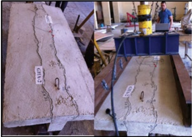
Figure 11. Cracks pattern of specimen GIIA-2.
