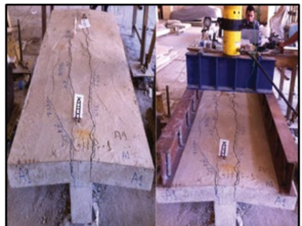
Figure 10. Cracks pattern of specimen GIIA-1.
