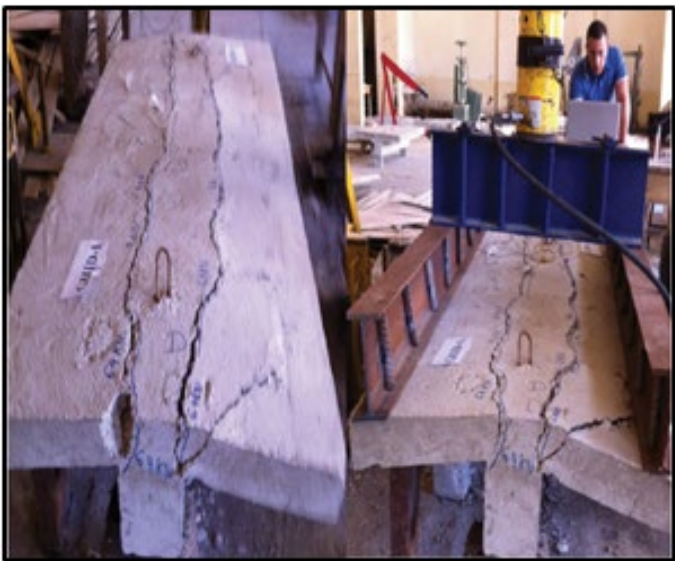
Figure 12. Cracks pattern of specimen GIIID-1.
