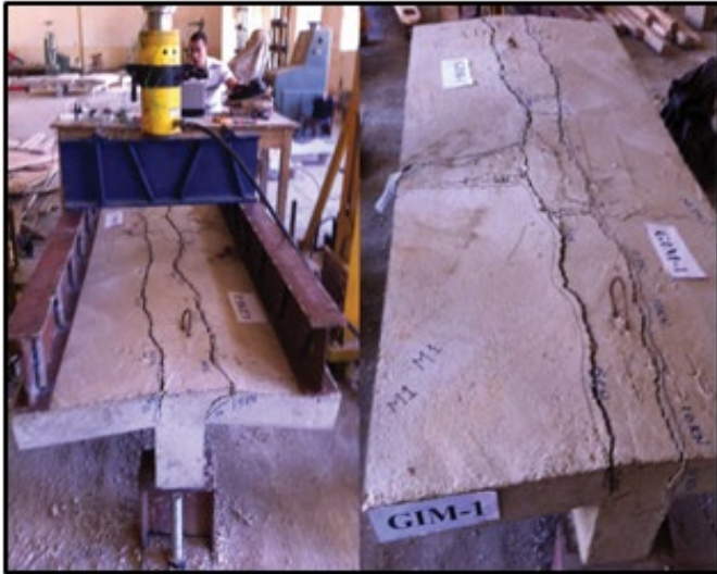
Figure 6. Cracks pattern of specimen GIM-1.
