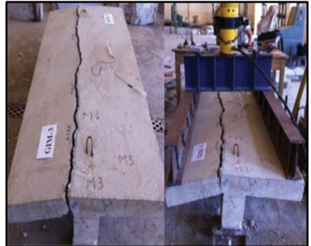
Figure 8. Cracks pattern of specimen GIM-3.
