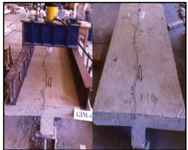
Figure 9. Cracks pattern of specimen GIM-4.
