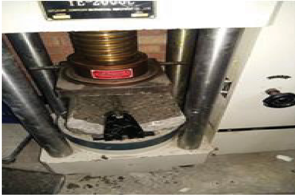
Figure 8. Split tensile strength test setup.
