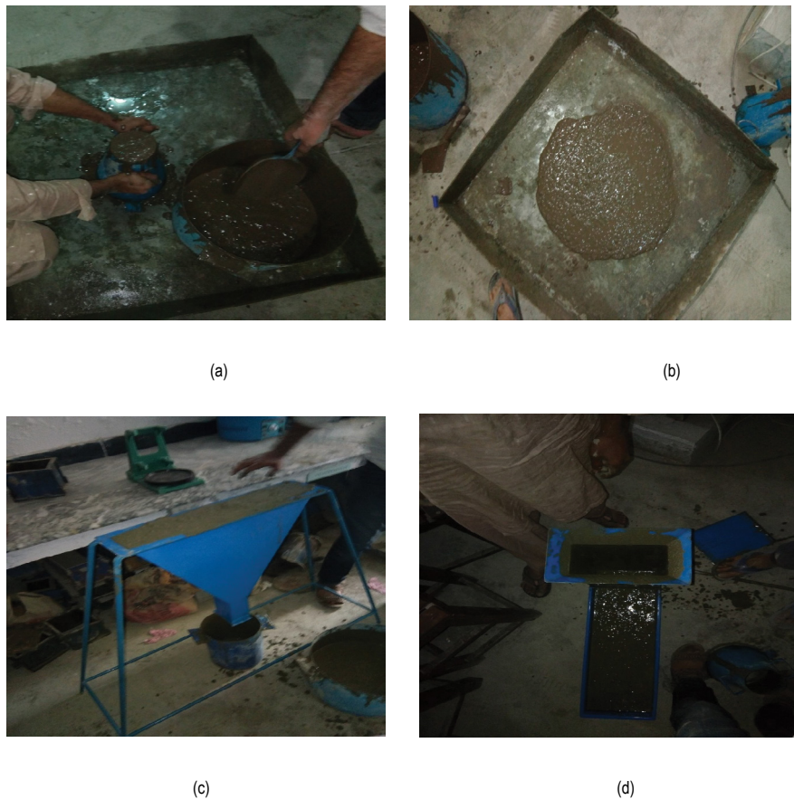
Figure 1. (a), (b) Slump flow, (c) V- funnel, (d) L- box tests.
