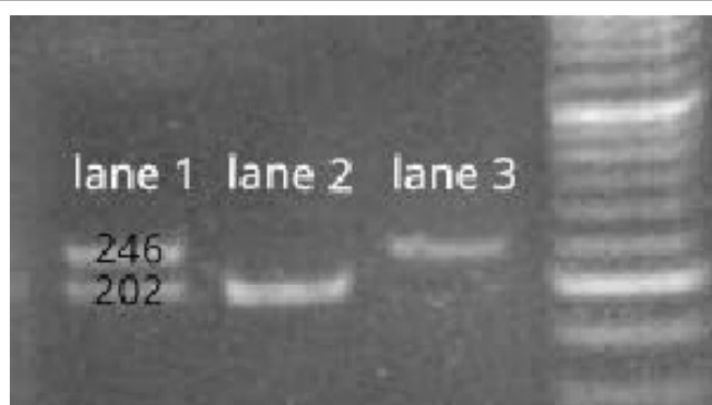
Figure 1: Electrophoresis image of the ESR1 genotyping visualized by ethidium bromide staining on agarose gel. The lengths of the DNA fragments are (1) 246 bp and 202 bp for the TC genotype, (2) 202 bp for the TT genotype (3) 246 bp for the CC genotype.(44 bp couldn't be seen).
