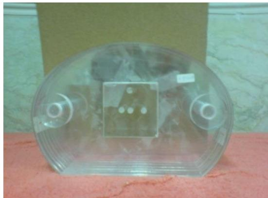
Figure 4: Phantom for Monte Carlo validation.
