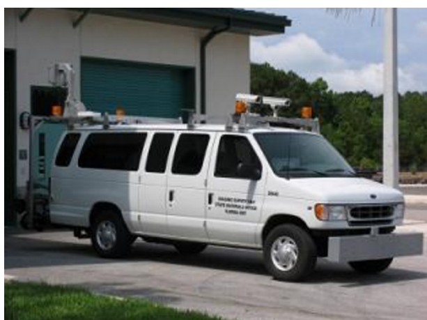
Figure 1: Survey van used for IRI data Collection Florida DOT.
