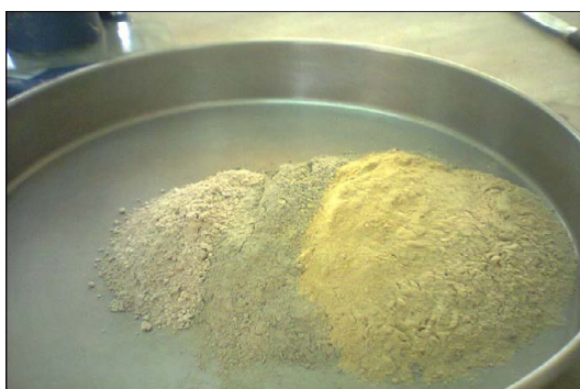
Figure 2: A sample containing limestone, coal ash and OPC (before blending).
