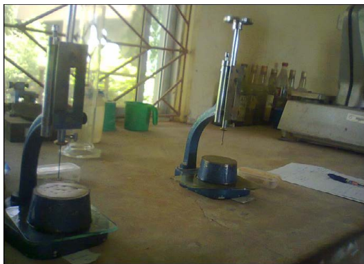
Figure 3: Experimental setup for Initial setting time test with Vicat needle (A) and final setting time test with Vicat needle + annular attachment (B).
