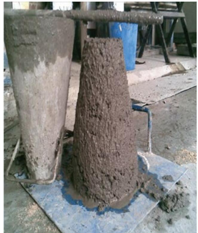
Figure 4. Slump test.
