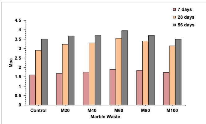
Figure 11. Flexure strength results.
