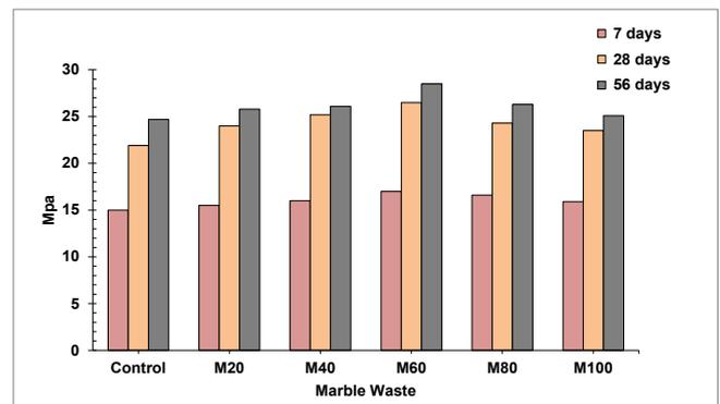
Figure 9. Split tensile strength results.
