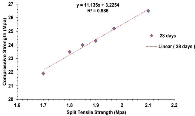
Figure 10. Co - relation between compressive and split tensile strength.
