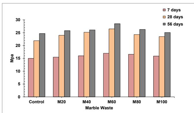
Figure 7. Compressive strength results.
