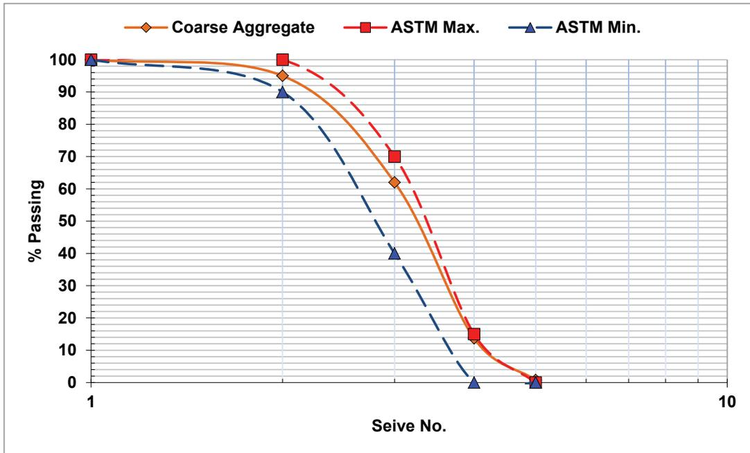
Figure 2. Gradation curve coarse aggregate.
