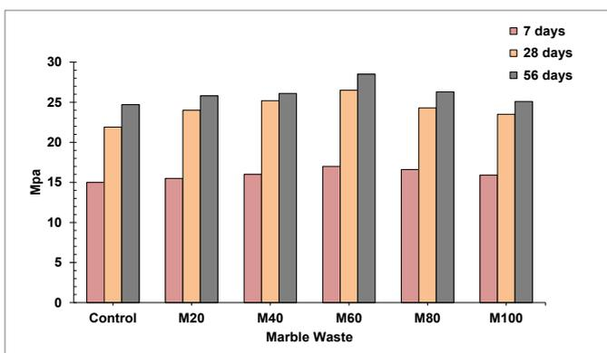
Figure 7. Compressive strength results.
