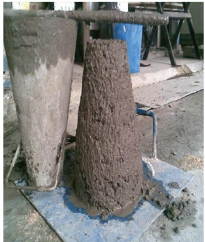
Figure 4. Slump test.
