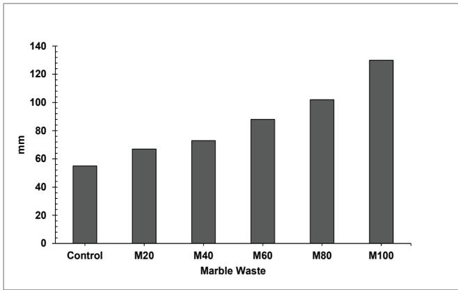
Figure 5. Slump test results.
