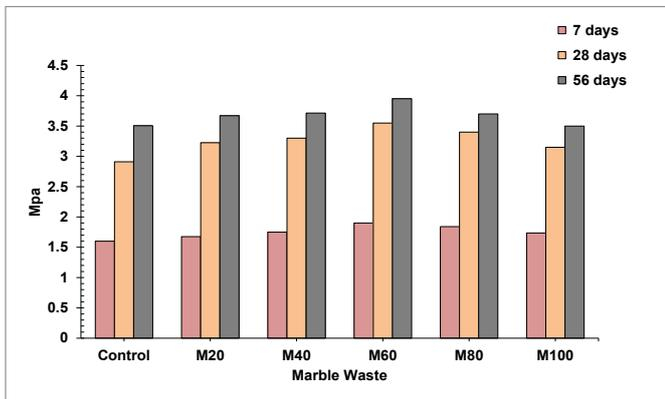
Figure 11. Flexure strength results.
