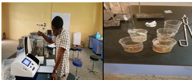
Figure 10. Taking readings from the Photometer and samples before the readings are taken.
