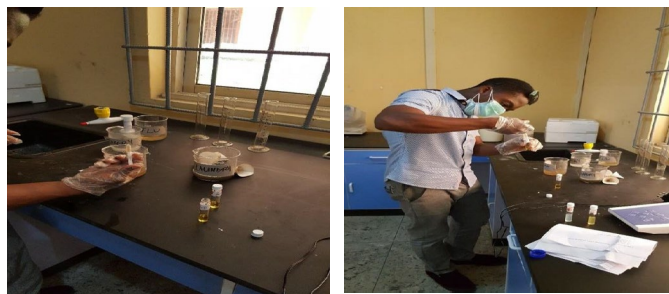
Figure 9. Ensuring that there was no bubble and inserting the sample in the COD bottle.
