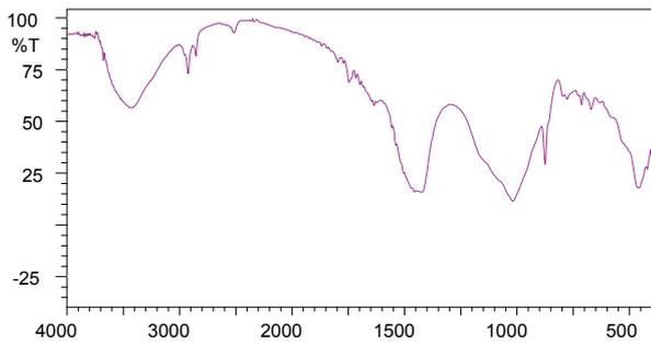
Figure 13. FTIR spectra of CO<sub>2</sub> absorption.
