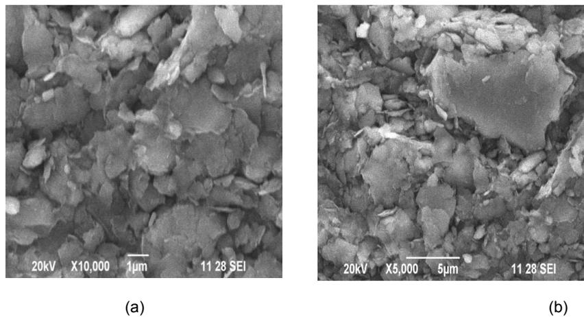
Figure 7. Scanning Electron Microscope (SEM) surface image of zeolite with magnification. (a) 10000x and (b). 5000x SEM view of zeolite in different focus.
