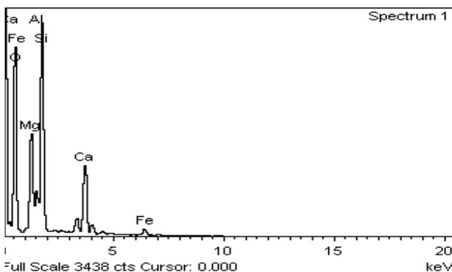
Figure 8. Composition of elements in zeolite.
