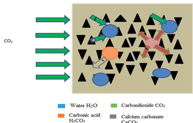
Figure 2. Carbonation in concrete.
