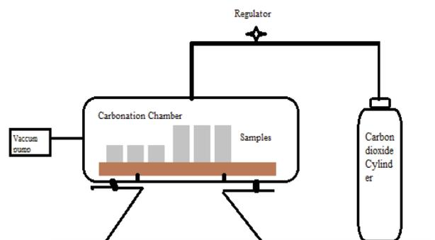
Figure 6. Carbonation chamber model.
