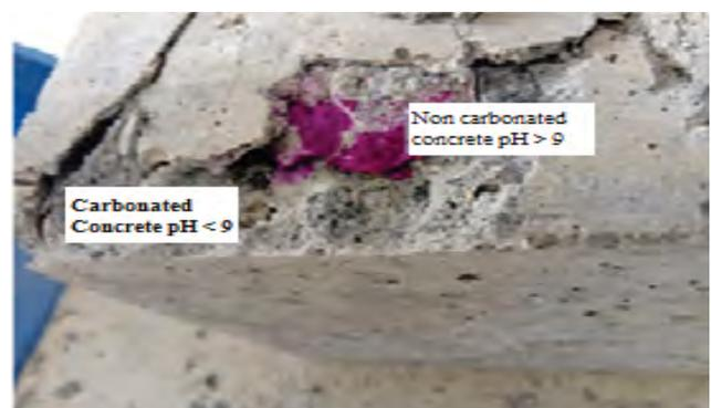
**Figure 12.** Degree of carbonation.
