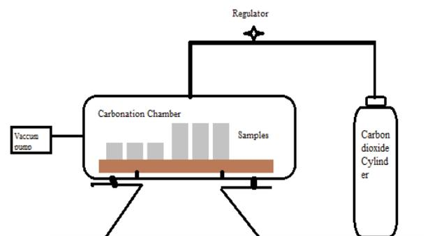
Figure 6. Carbonation chamber model.
