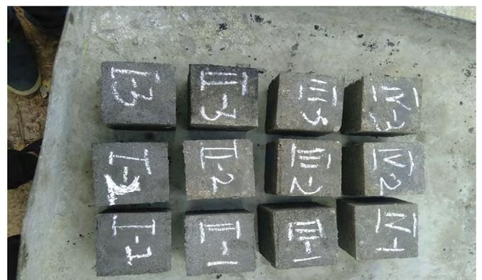
Figure 9. Cement mortar cube specimen.
