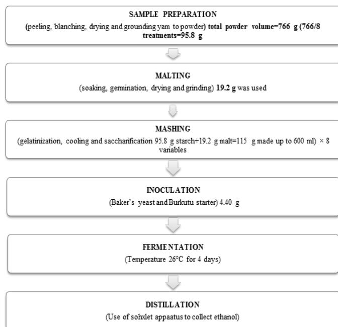
A sohxlet apparatus was used to collect the ethanol obtained by the processes above.
