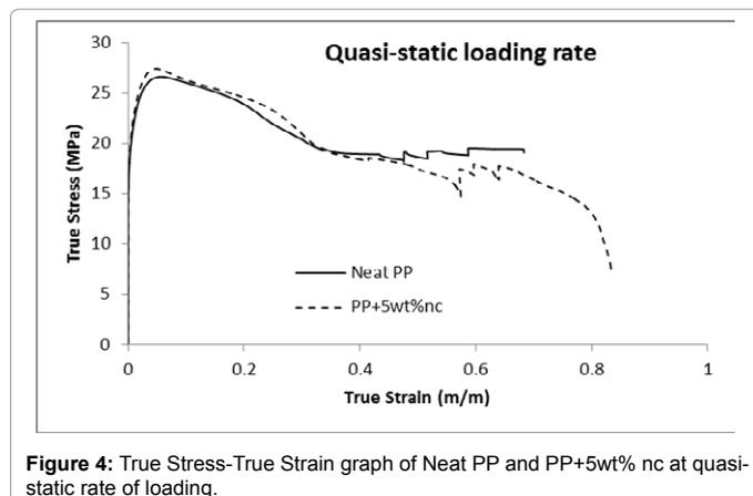
Figure 4: True Stress-True Strain graph of Neat PP and PP+5wt% nc at quasi-static rate of loading.
