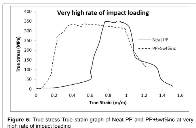
Figure 5: True stress-True strain graph of Neat PP and PP+5wt%nc at very high rate of impact loading
