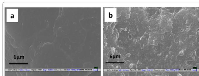
Figure 3: SEM images of specimens before loading (Mag. 10kX) (a) Neat PP (b) PP+5wt%nc.
