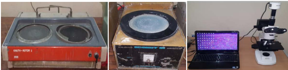
Figure 3: (a) Electric disk rotary grinding, (b) polishing device (c) optical microscope for microstructure observation.
