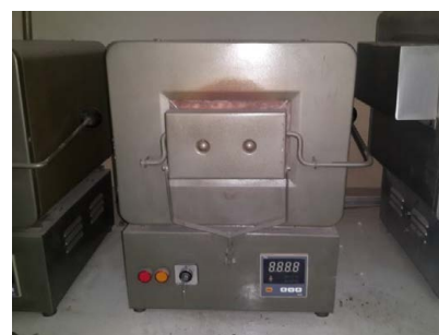
Figure 2: Electric resistance box furnace type for aging samples.
