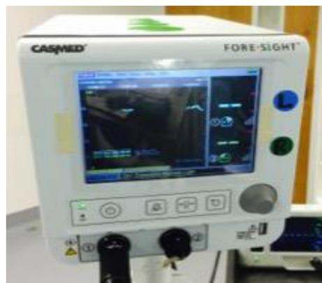
Figure 2a: CASMED device unable to obtain reading due to 'Excessive Ambient Light'. Note error reading at bottom of screen.
