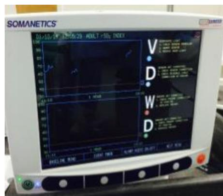
Figure 2b: INVOS device reading error demonstrated to the right of row marked by 'V'.
