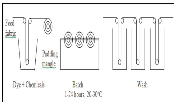
Figure 1. Pad-batch method.
