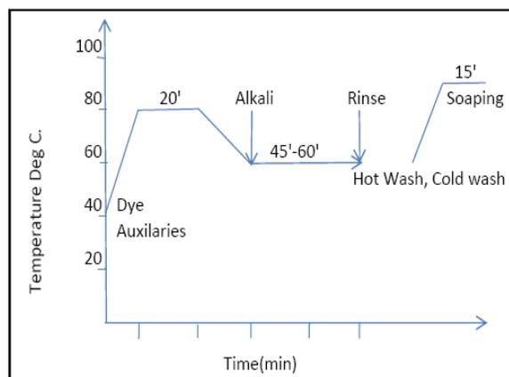
**Figure 3.** Process flow of Novacron Brilliant Blue H-GR.
