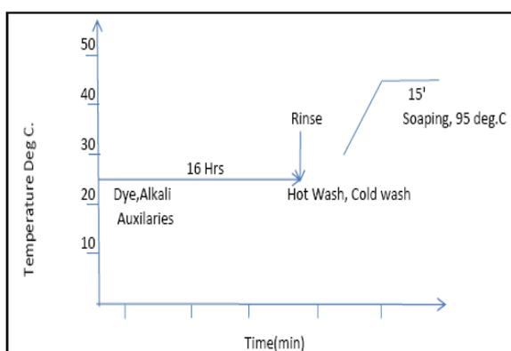
**Figure 2.** Process flow of pad batch dyeing.
