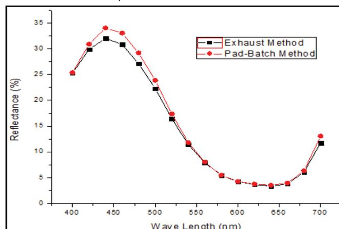
**Figure 4.** Reflectance value of Novacron Brilliant Blue H-GR.
