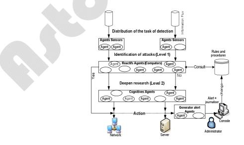
Figure 1. Proposed platform of intrusion détection.
