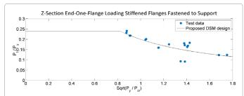
Figure 6: Comparison of DSM curves with the test data for Z-section EOF loading condition.
