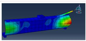
Figure 4: Web crippling of a Z-section stiffened flanges subjected to End-One-Flange loading.
