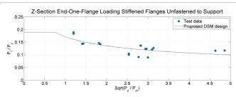
Figure 7: Comparison of DSM curves with test data for Z-section EOF loading condition.
