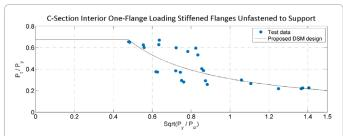
Figure 5: Comparison of DSM curves with test data for C-section IOF loading condition.
