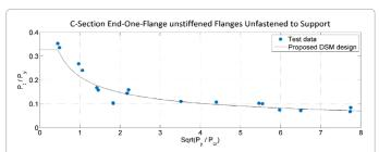
Figure 10: Comparison of DSM curves with test data for C-section EOF loading
