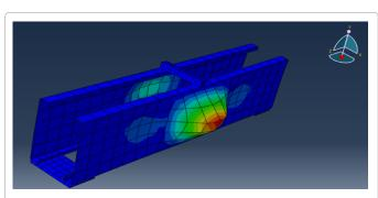
Figure 3: Web crippling of CFS C-section (stiffened flanges) subjected to Interior One-Flange loading.
