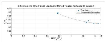
Figure 8: Comparison of C-section End-one-flange Loading DSM curves with the test data
