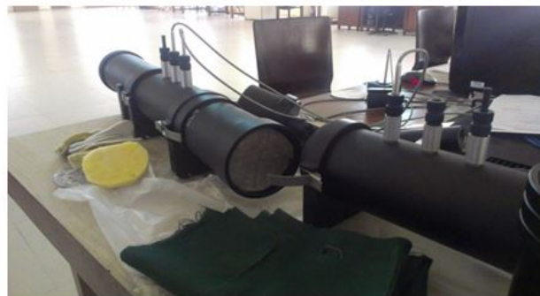
Figure 2: Impedance Tube Method (ASTM E 1050).
