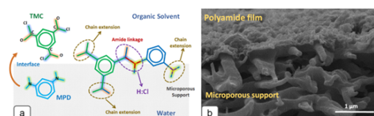
Figure 2. (a) illustration of interfacial polymerization reaction between MPD and TMC monomers, (b) cross-sectional images of the TFC membrane having a thin polyamide layer over a porous support membrane.
