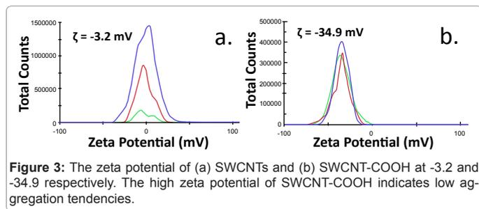
**Figure 3:** The zeta potential of (a) SWCNTs and (b) SWCNT-COOH at -3.2 and -34.9 respectively. The high zeta potential of SWCNT-COOH indicates low aggregation tendencies.
