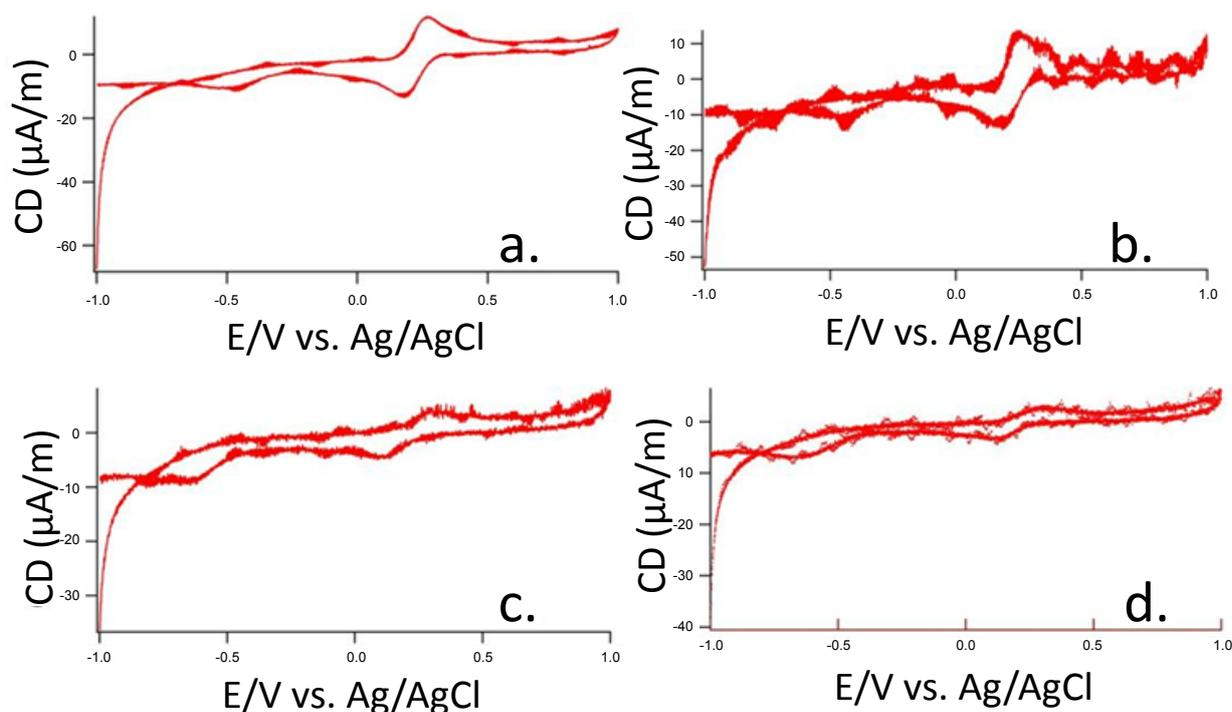
**Figure 8:** Cyclic Voltammetry the GC electrode in the presence of 0.5mM Fe (CN) 6<sup>-3</sup>/ Fe (CN)6<sup>-4</sup> (scan rate 100.0 mVs<sup>-1</sup>); (a) bare GC electrode (b) after functionalization with SWCNT-COOH (c) after immobilization of SWCNT-antibody (d) after the formation of antigen-antibody complex.
