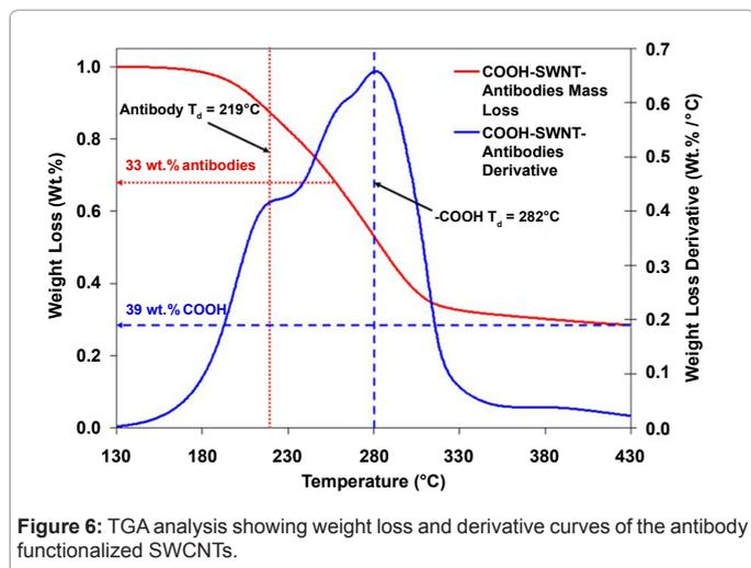
**Figure 6:** TGA analysis showing weight loss and derivative curves of the antibody functionalized SWCNTs.
