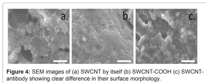
**Figure 4:** SEM images of (a) SWCNT by itself (b) SWCNT-COOH (c) SWCNT-antibody showing clear difference in their surface morphology.
