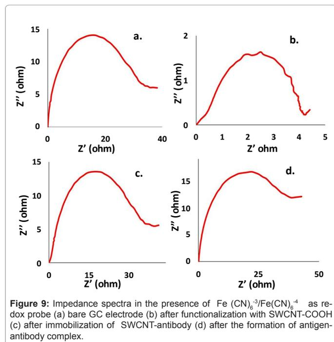
**Figure 9:** Impedance spectra in the presence of  $\text{Fe}(\text{CN})_6^{3-}/\text{Fe}(\text{CN})_6^{4-}$  as redox probe (a) bare GC electrode (b) after functionalization with SWCNT-COOH (c) after immobilization of SWCNT-antibody (d) after the formation of antigen-antibody complex.
