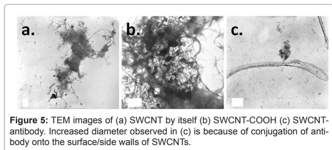
**Figure 5:** TEM images of (a) SWCNT by itself (b) SWCNT-COOH (c) SWCNT-antibody. Increased diameter observed in (c) is because of conjugation of antibody onto the surface/side walls of SWCNTs.
