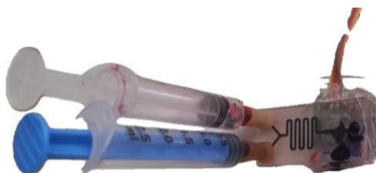
Figure 18. Red and blue ink mixing Y channel serpentine mixer with chamber for 2 inlet and 1 outlet.
