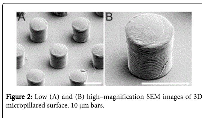
**Figure 2:** Low (A) and (B) high-magnification SEM images of 3D micropillared surface. 10 μm bars.
