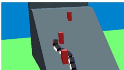
Figure 3: Terrain for developing intelligent lateral control of the OT-4 model in the Yobotics! Simulation Construction Set.
