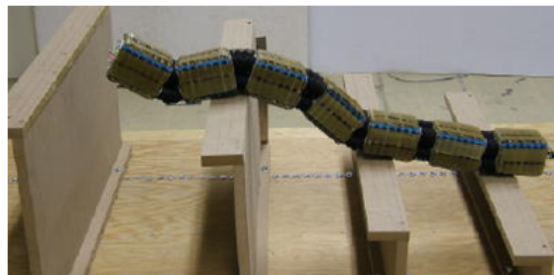
Figure 1: The Omni Tread OT-4 serpentine robot climbing over parallel bars under automated control.
