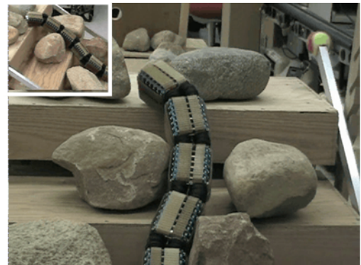
Figure 2: The Omni Tread OT-4 robot on stairs terrain with rocks, requiring control of sagittal and lateral movements.
