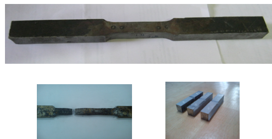
Figure 1: Test samples of tensile and impact.
