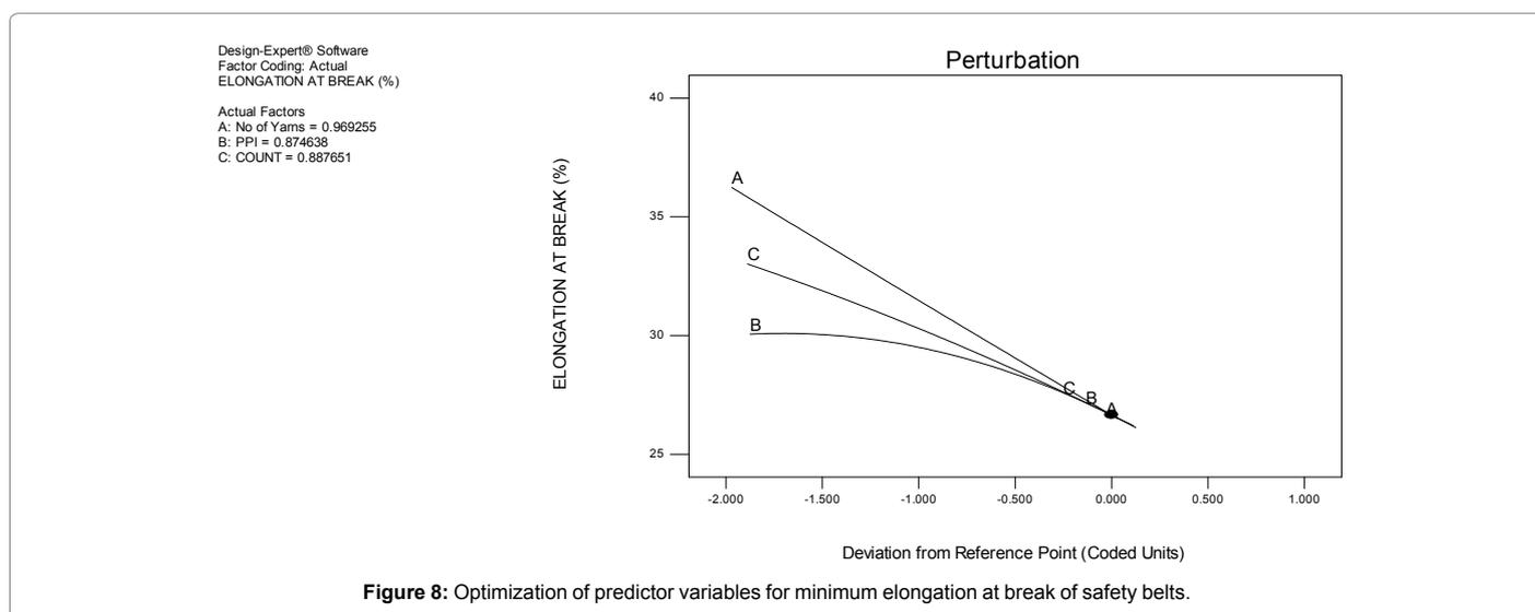
Figure 8: Optimization of predictor variables for minimum elongation at break of safety belts.
