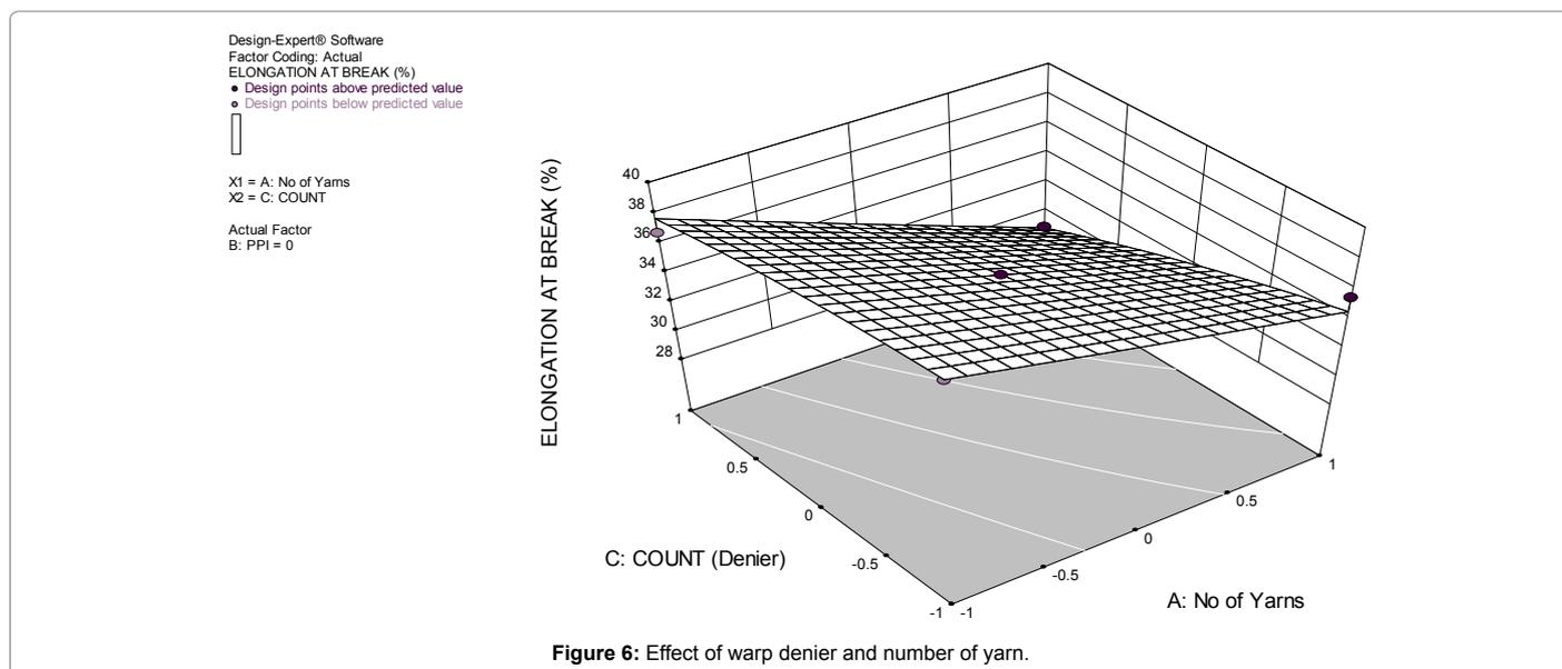
effect on the elongation at break of the safety belt. The elongation at break of safety belts reduces with increase in the number of warp yarns. The relation is linear as depicted by the analysis of variance and the Figure 6. The reason behind this is that the higher denier will have the more number of filaments in the warp direction and consequently will have more load bearing capacity and hence low elongation at break. Effect of warp denier is more pronounced at higher number of yarns.
