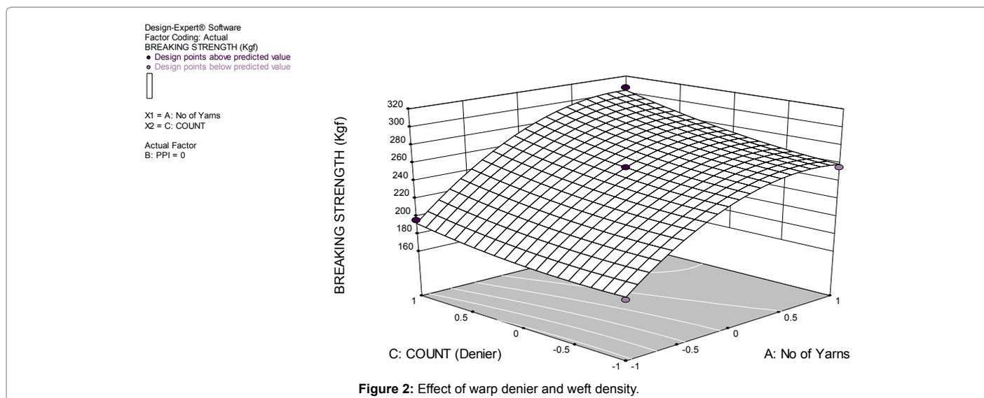
effect on the breaking strength of the safety belt. But the effect is relatively low as compared to the effect of number of yarns. Breaking strength of safety belts increases with increase in the denier of warp yarns. The relation is linear in this case as depicted by the analysis of variance and the Figure 2. The reason behind this is that the higher denier will have the more number of filaments in the warp direction and consequently will have more load bearing capacity.
