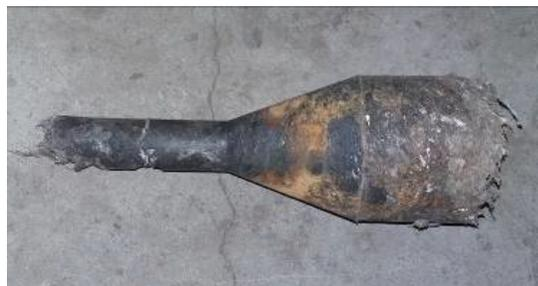
Figure 8: Stopper plug extracted from the draw die.
