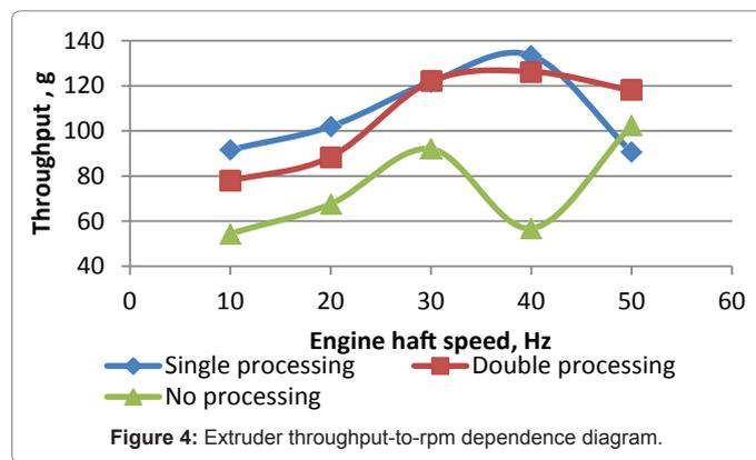
Figure 4: Extruder throughput-to-rpm dependence diagram.
