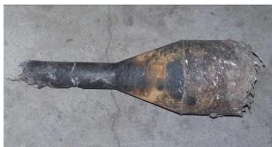
Figure 8: Stopper plug extracted from the draw die.
