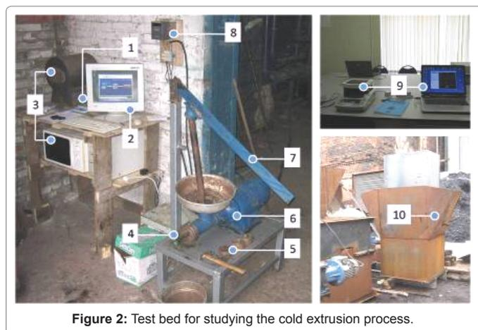
Figure 2: Test bed for studying the cold extrusion process.
