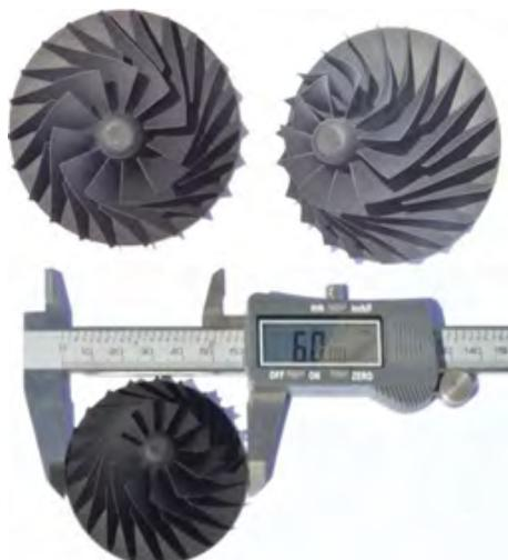
Figure 7. A 3-D printed plastic impeller of developed design of a miniature axial-centrifugal flow pump with 60 mm impeller blades diameter.
