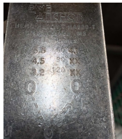
Figure 2: Lifting sling instructions plate.
