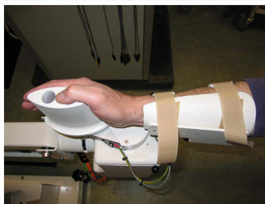
Figure 9: Top-view of the Wristalyzer®, (MOOG, Nieuw Vennep, the Netherlands).
