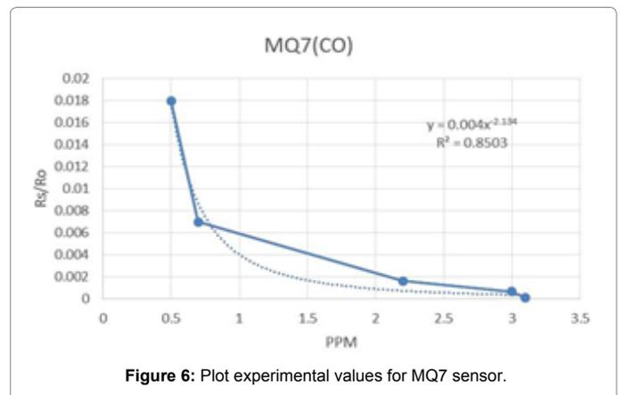
Figure 6: Plot experimental values for MQ7 sensor.
