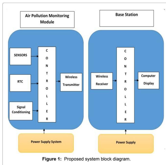
Figure 1: Proposed system block diagram.
