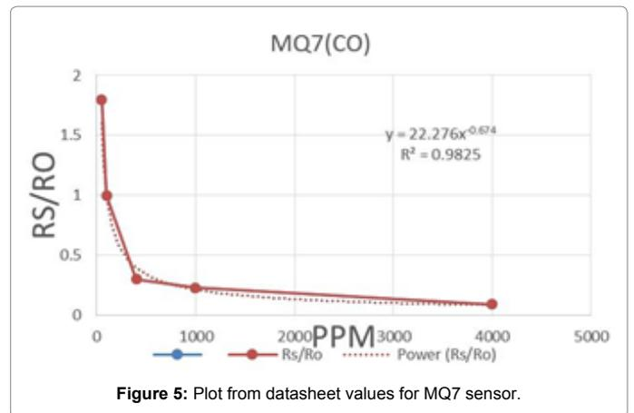
Figure 5: Plot from datasheet values for MQ7 sensor.
