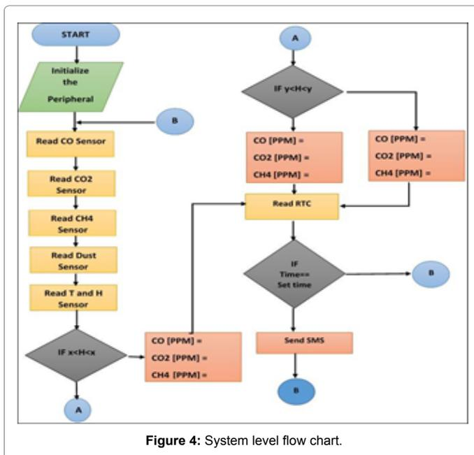
Figure 4: System level flow chart.
