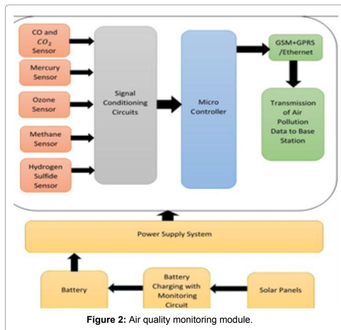
Figure 2: Air quality monitoring module.
