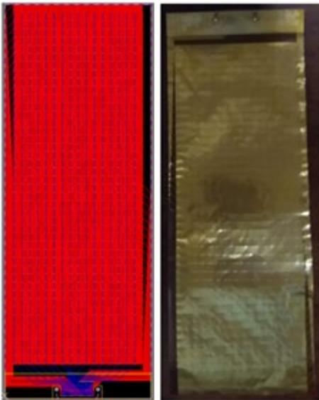
**Figure 2.** Sensor bed traces (left), manufactured sensor bed (right)
