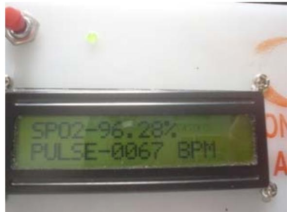
Figure 8: LCD display showing SpO<sub>2</sub> and Pulse Rate
