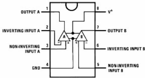
Figure 4: Low Power Dual Operational Amplifier LM358
