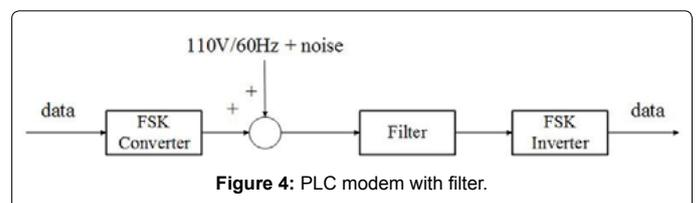
Figure 4: PLC modem with filter.
