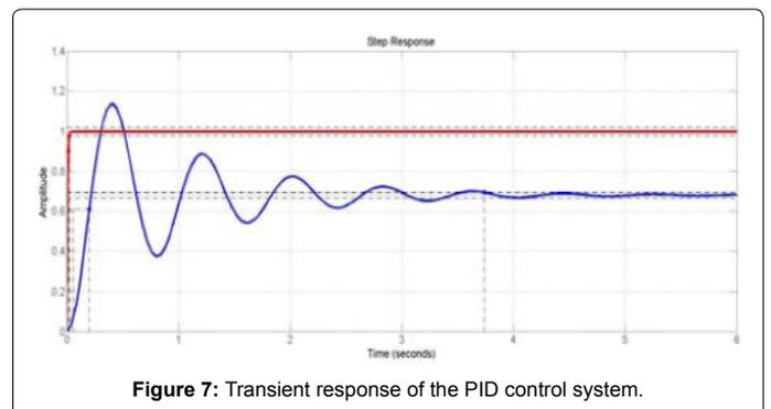
Figure 7: Transient response of the PID control system.
