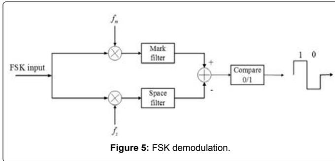
Figure 5: FSK demodulation.
