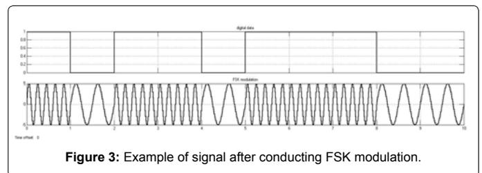
Figure 3: Example of signal after conducting FSK modulation.
