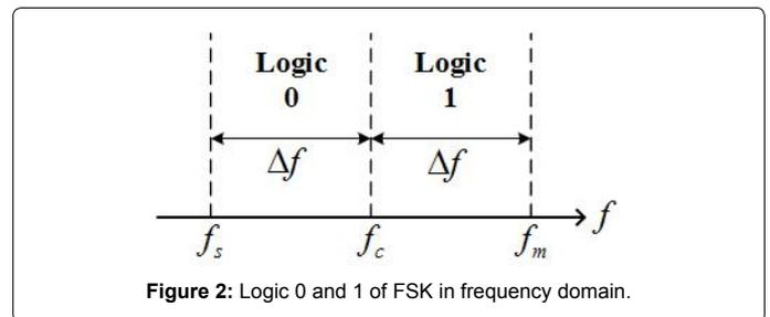
Figure 2: Logic 0 and 1 of FSK in frequency domain.
