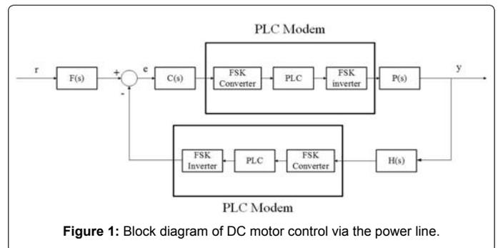
Figure 1: Block diagram of DC motor control via the power line.
