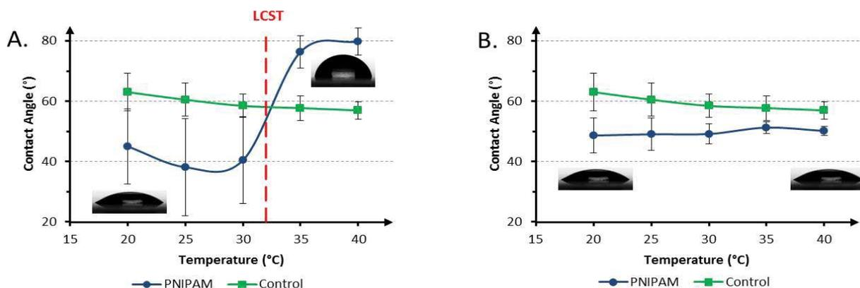
**Figure 3:** Static contact angle measurement versus temperature after first use (A) and after several uses (B) of the PNIPAM-grafted chips for cell detachment. For each curve, 3 substrates were used, and 9 measurements were performed on each substrate in different locations for any given temperature. Thermal behavior of PNIPAM-grafted (green) and bare glass slides (Ctrl, blue). LCST: Lower critical solution temperature.
