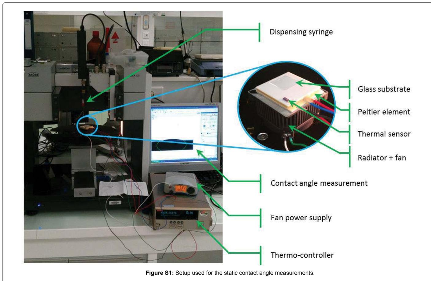
Figure S1: Setup used for the static contact angle measurements.
