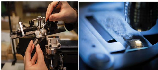
Figure 4: Preparation (microtome) and microscopic analysis of wood sections.
