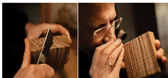
Figure 1: Preparation of the transverse plane and macroscopic observation of the wood structures.
