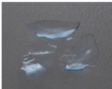
Figure 2: Acuvue 2 contact lens fractured into fragments after dehydration.
