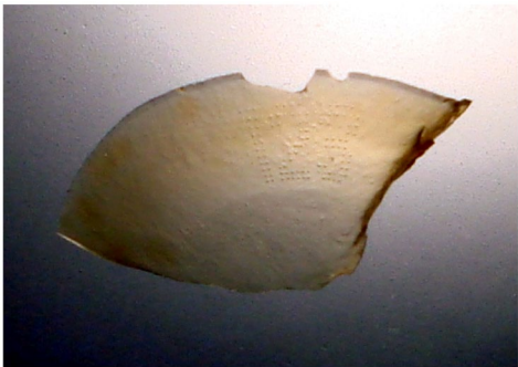
Figure 6: Sample A was the critical piece of evidence that convicted Raven Abaroa. Note inversion marks labeled 123, that identified the remnant as a Vistakon Acuvue 2® contact lens.
